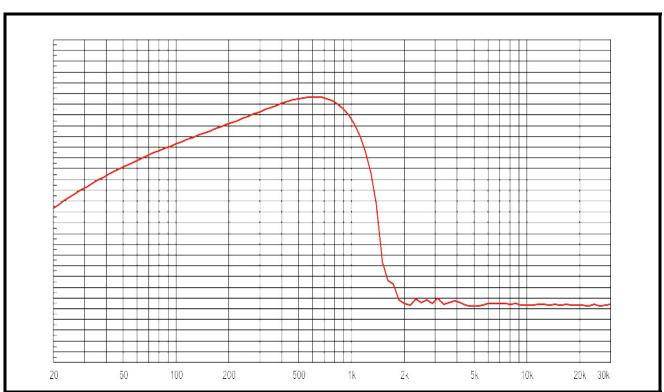
FIGURE 27. Frequency Response - Preset 2 (300Hz to 900Hz)
